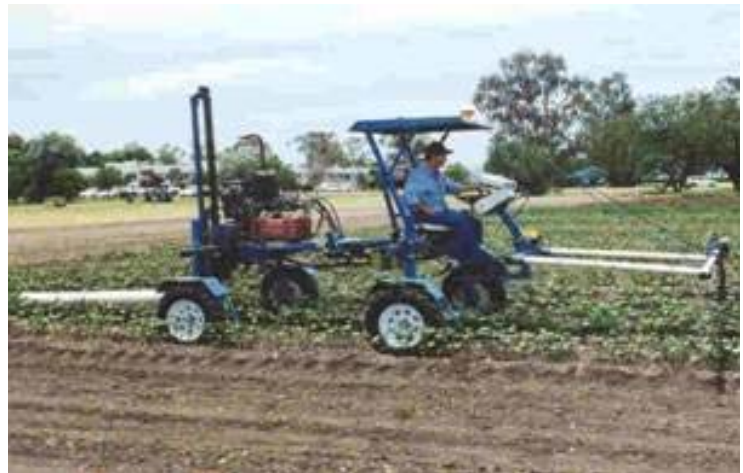
The Mobile Electromagnetic Sensing System (MESS) used to undertake electromagnetic (EM) surveys
